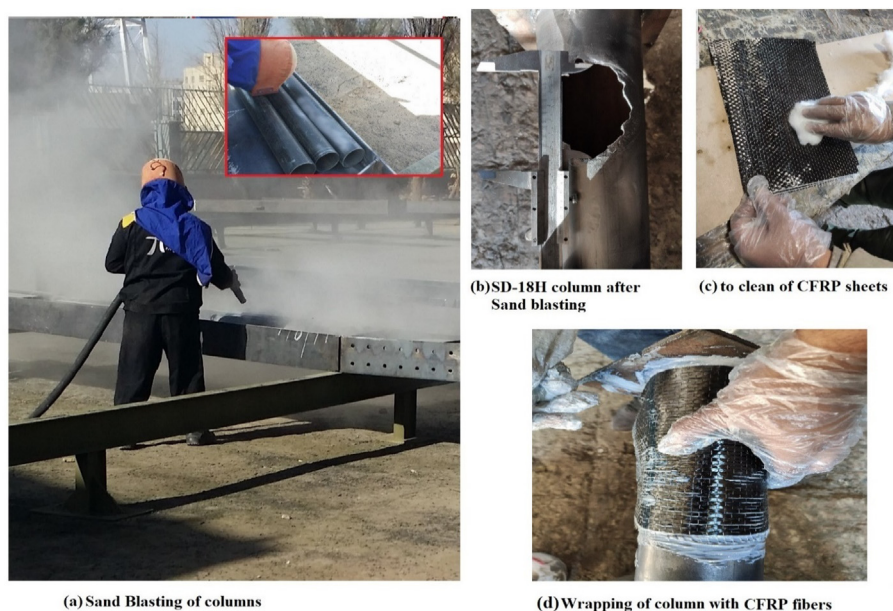
Fig. 9. Preparing CFRP-strengthened specimens.
