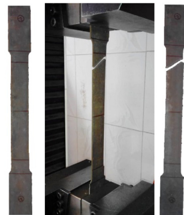
Fig. 2. Tensile test and the failure mechanism.
