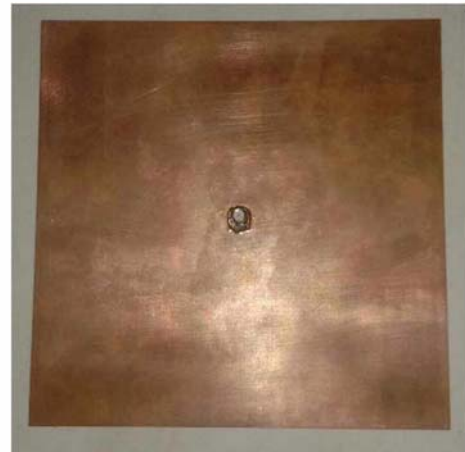
Fig. 7. The bottom layer of fabricated 4x4 microstrip patch array antenna
