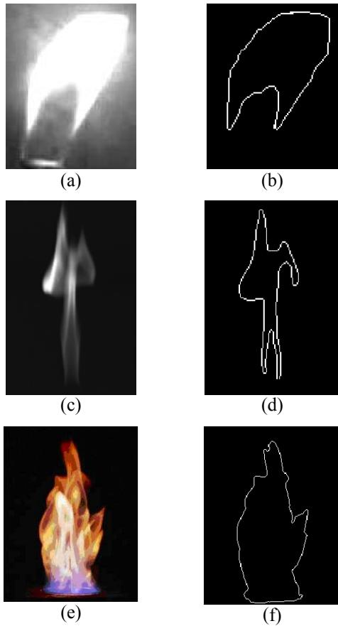
Figure 4. Some of the flame edge detection results [Left column: original images; right column: images with identified edges. (a) Diffusion pronane-flame, (c) Partially-premixed pronane-flame, (e) Small scale pool fire[13]].
