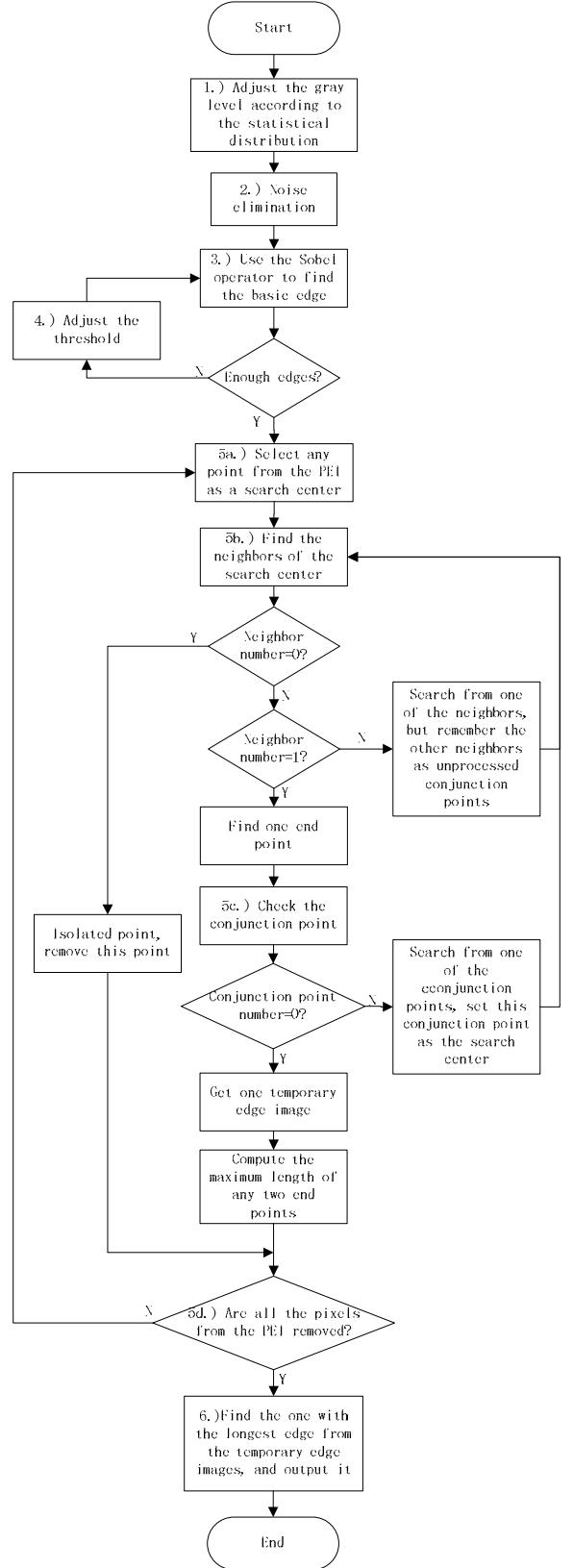
Figure 3. Flow chart of the flame edge detection algorithm.
