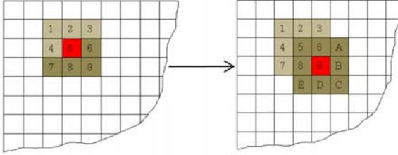
Figure 2. Illustration of movement of the edge search.
