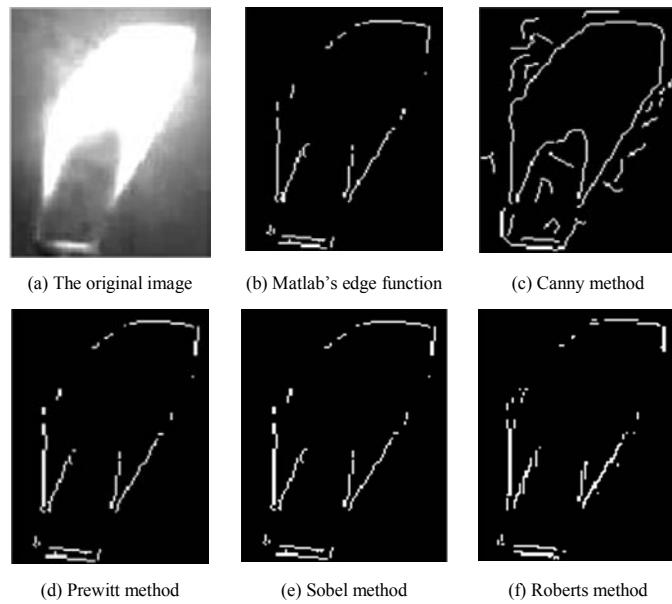
Figure 1. Representative results using the common edge detection methods.
